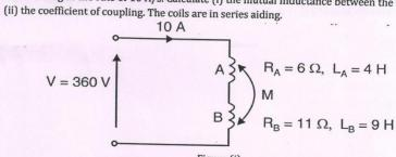
$\label{eq:Figure} Figure~(i)$  Find the equivalent inductance  $L_{AB}$  in Figure (ii). Make necessary assumptions if required. [05]
